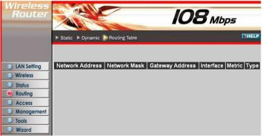
Network Address: Displays the network IP address of the connected node. Network Mask: Displays the network (subnet) mask of the connected node. Gateway Address: Displays the gateway address of the connected node. Interface: Displays whether the node is connected via a WAN or LAN. Metric: Displays the metric of the connected node.
